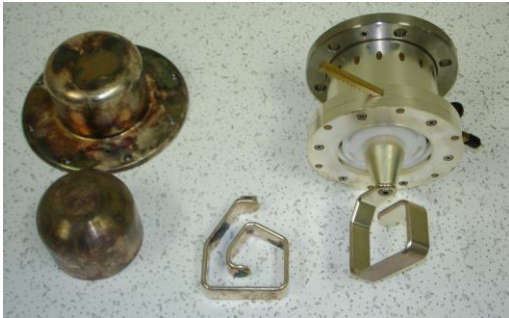
FIGURE 2 IOT CAVITY COUPLING LOOPS & DOMES (E2V)
