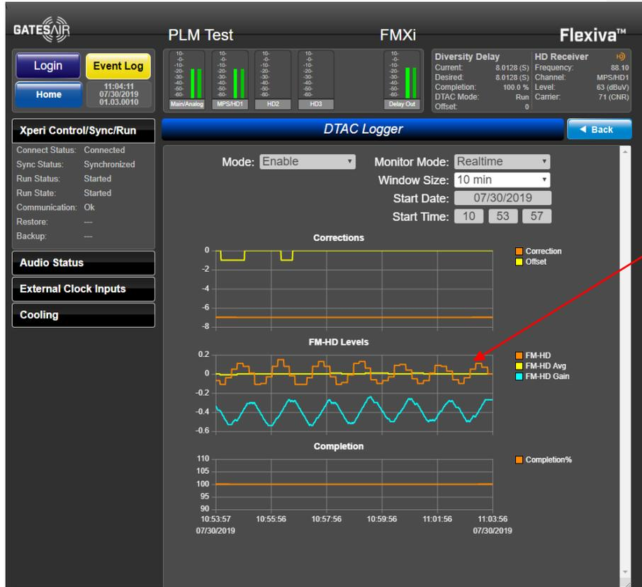
Realtime monitoring and logging of DTAC corrections and levels
