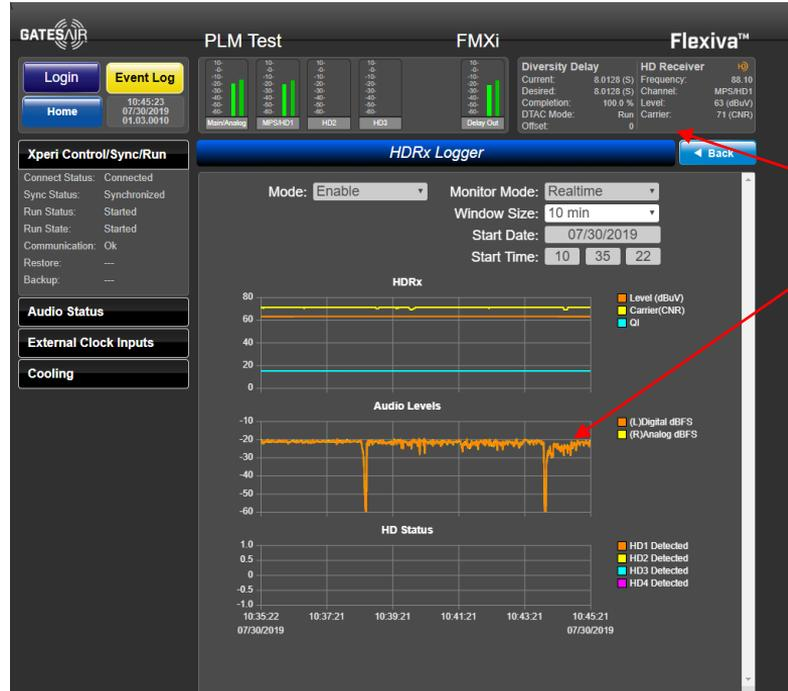
Realtime monitoring FM Signal and HD Carrier to Noise ratio
