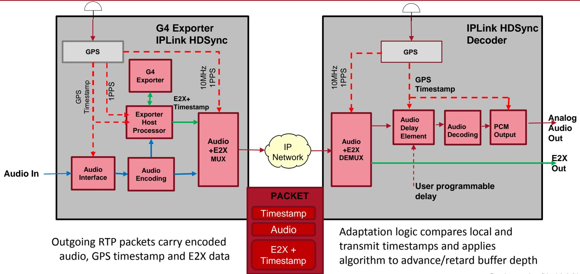
Outgoing RTP packets carry encoded audio, GPS timestamp and E2X data
