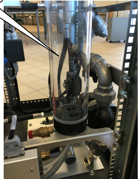
Automatic Liquid Refilling System (8 litres capacity)
