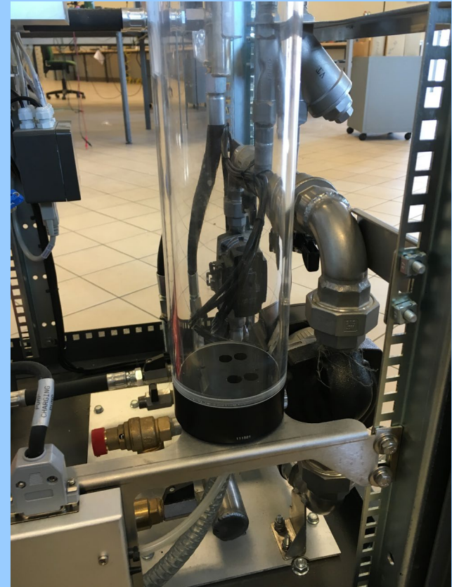
Automatic Liquid Refilling System (8 litres capacity)
